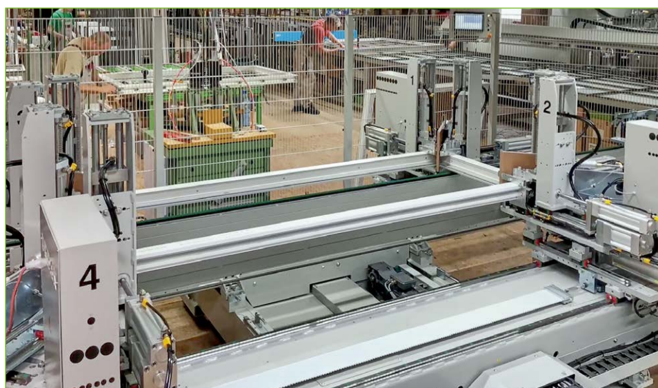
The AKS 6410/4 from RB Reinert changes the fixtures automatically.
